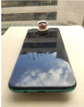
Fig. 5a Take zenith photo with fish eye lens (wide angle lens).
